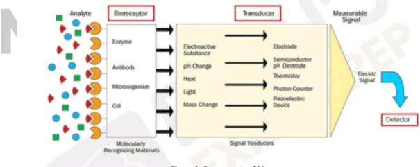
Figure 1. Components of biosensor
