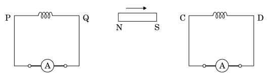
A bar magnet is moved in the direction indicated by the arrow between two coils PQ and CD. Predict the direction of the induced current in each coil.
