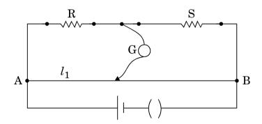
An unknown resistance X is now connected in parallel to the resistance S and the balance point is found at a distance  $l_2$ . Obtain a formula for X in terms of  $l_1$ ,  $l_2$  and S.
