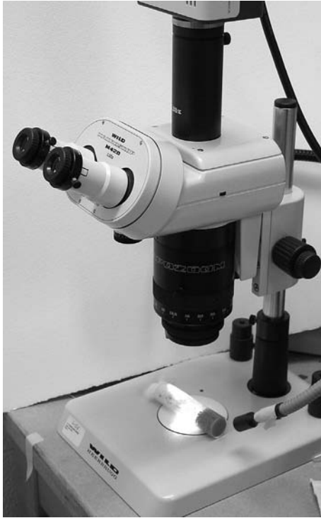
Fig. 4.6 A research-grade stereomicroscope. Note the light source is from the side, which can give a shadow effect to the specimen; in this example a vial of fruit flies. The large objective lens above the specimen can be rotated to zoom the image.
