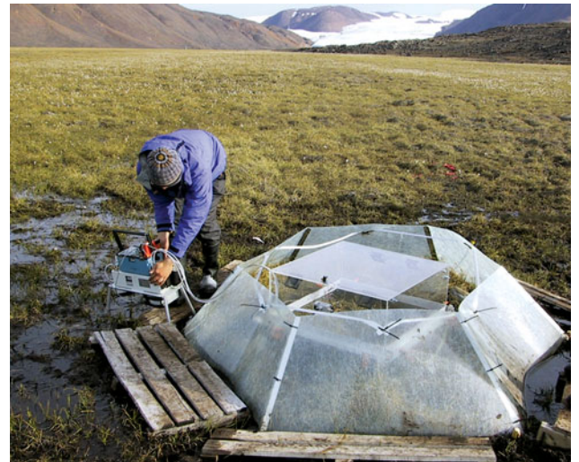
Figure 30.19 The International Tundra Experiment (ITEX) uses small, passive, clear plastic, open-top chambers to warm the tundra and extend the growing season. The chambers raise the daily temperature of the tundra plant canopy by 1.5^\circ\text{C} to 1.7^\circ\text{C} , which is in the range predicted by global climate simulations. This experiment, which has been in place in the Barrow Environmental Observatory for three years and for one year at Atkasuk, Alaska, has already provided new insights on flower and growth responses to warming.
